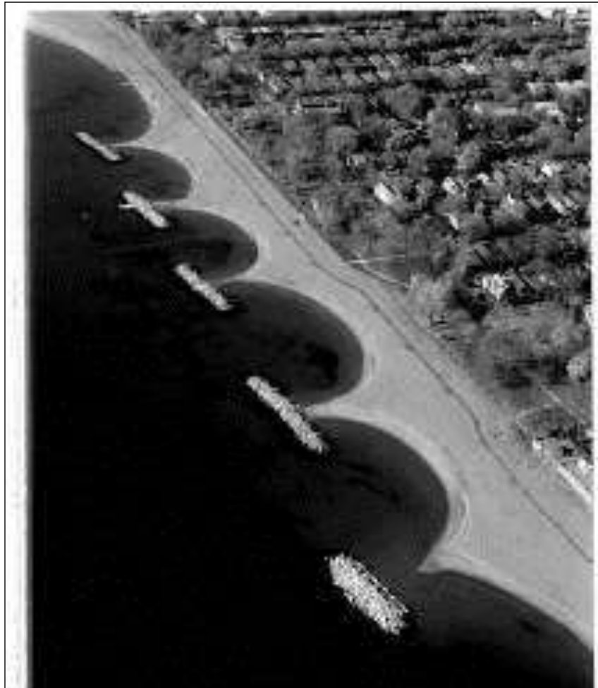
Figure 7.9 Example of erosion mitigation through shore-parallel structures (Anglin, et al. 2001)
