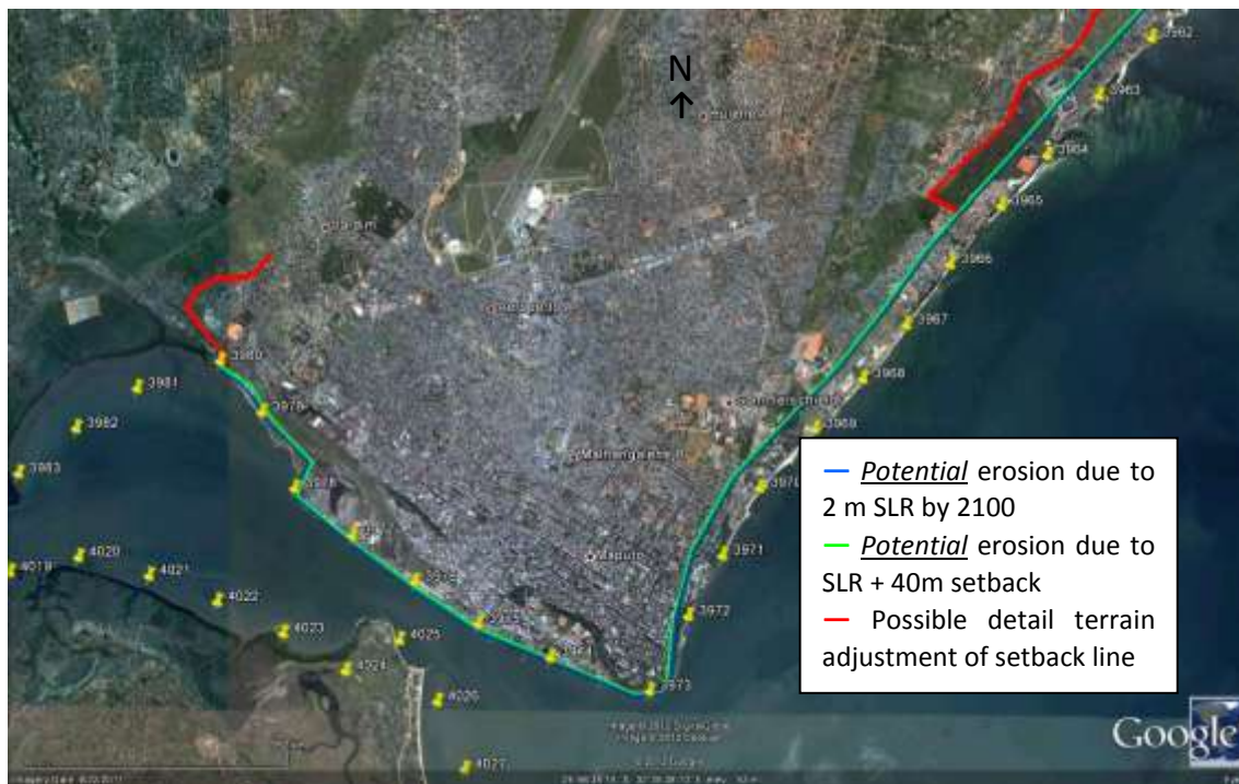
Figure 5.30: Map of potential erosion and setback line for SLR - Maputo
