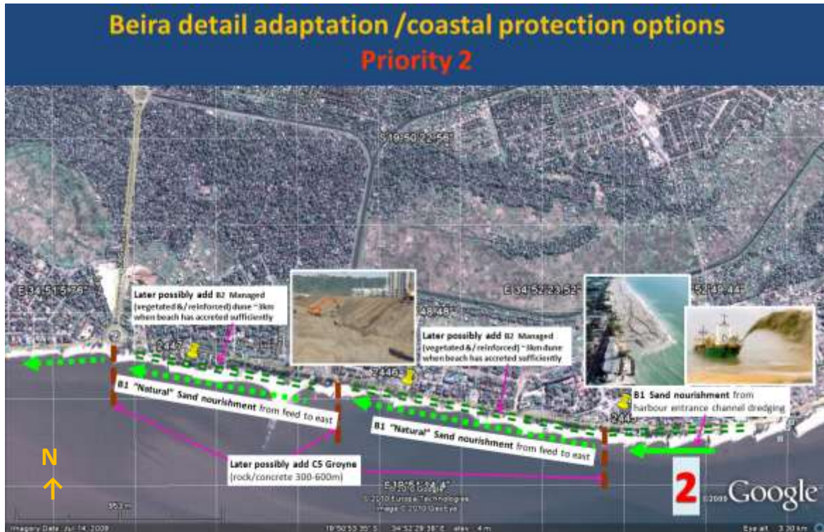
Figure 8.3: Southern Beira. Adaptation / coastal protection options based on general criteria, local site characteristics, current use/ "value".
